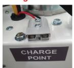
Easy Access Charger Port located on the machine frame.
